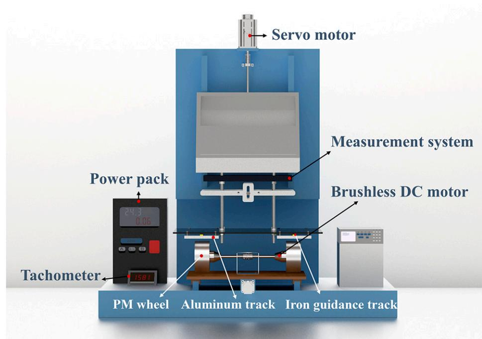
**Figure 18.** Schematic diagram of the annular PM EDS experimental prototype.
