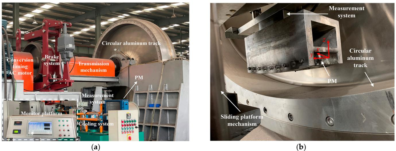
**Figure 4.** Photos of the PM EDS high-speed rotating experimental platform: (a) Overall schematic diagram of the device; (b) Schematic diagram of crucial parts.
