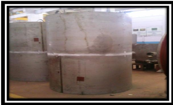
Figure 3. L-seam welding & DP test.
