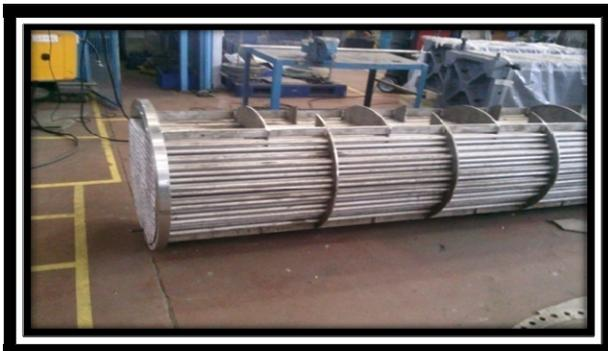
Figure 5. Tubes & Baffles assembly.
