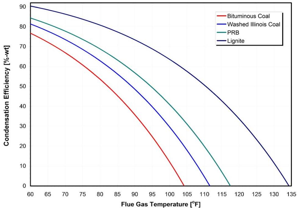
Figure 7. Condensing efficiency as a function of flue gas temperature.
