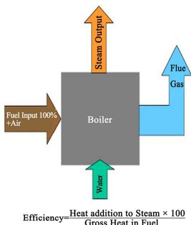
$$\text{Boiler Efficiency} = \frac{\text{Steam flow rate} \times (\text{steam enthalpy} - \text{feed water enthalpy})}{\text{Fuel firing rate} \times \text{Gross calorific value}} \times 100$$
