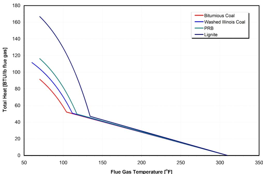
Figure 6. Flue gas heat vs gas temperature.
