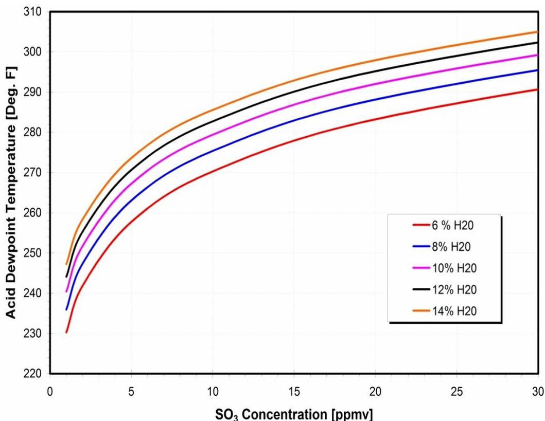
Figure 4. Acid dew point temperature as a function of the  $\text{SO}_3$  and  $\text{H}_2\text{O}$  concentration.
