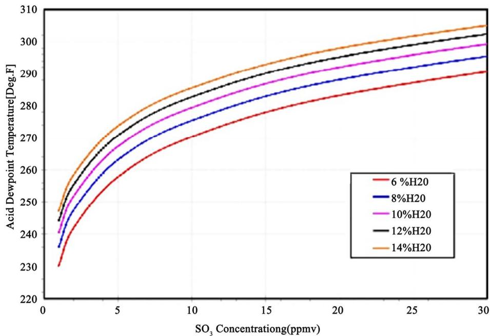
Figure 8. Acid dew point temperature vs condensation.
