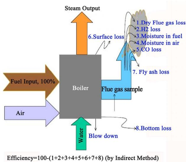
$$\text{Efficiency} = 100 - (1 + 2 + 3 + 4 + 5 + 6 + 7 + 8) \text{ (by Indirect Method)}$$
