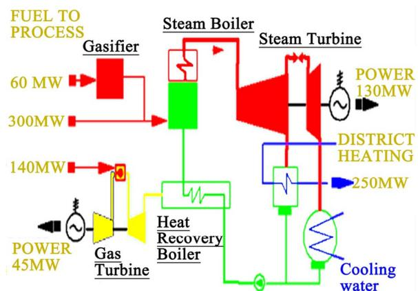
**Figure 1. Process flow chart of TPP.**
