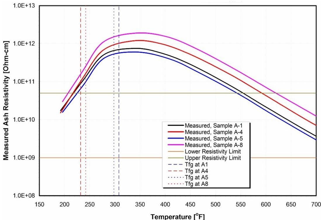
Figure 5. Ash resistivity versus flue gas temperature for a high-resistivity ash.
