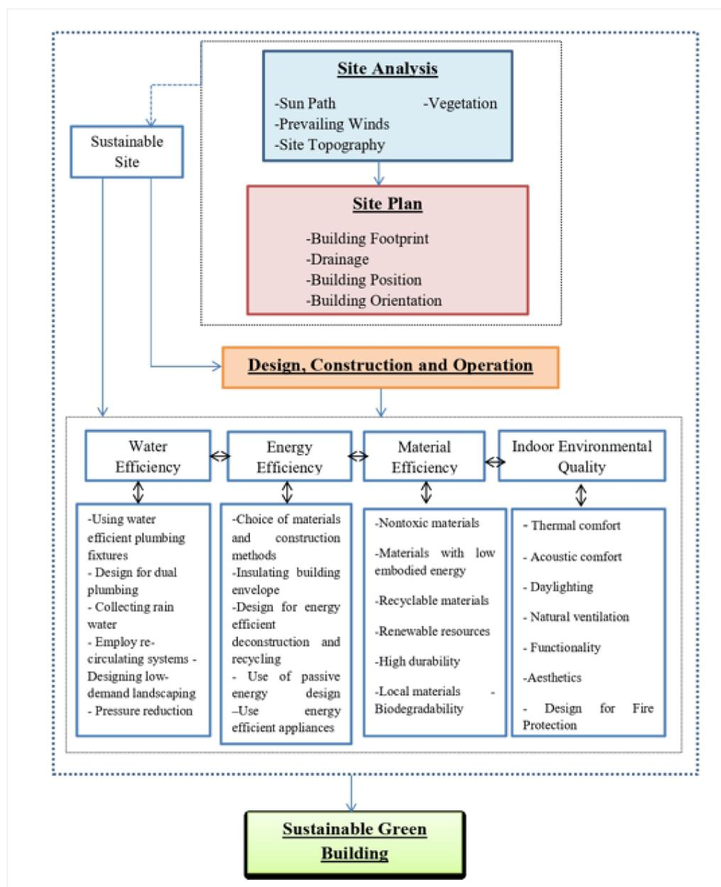
**Figure 6.** Framework for adopting the concepts and technologies of green building.
