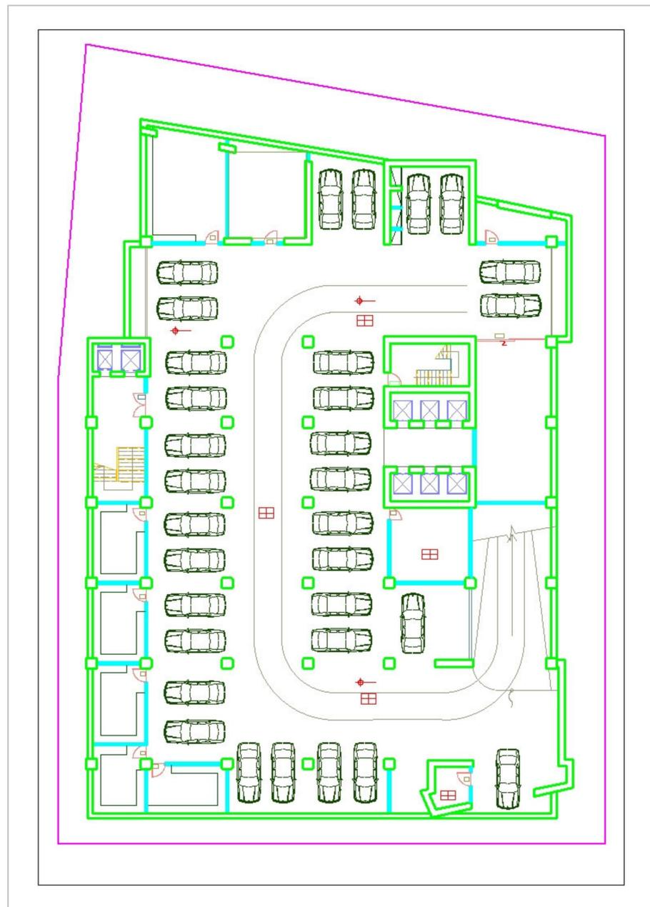
**Figure 3.** Floor plan for underground parking (source: ETG Designers and Consultants Sh.Co.).
